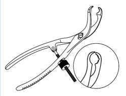
Allows bone to be held firmly in place whilst maintaining access to central area through gap between jaws.
