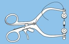
Stand alone instrument to add tension to line. Requires two extra crimps to add the tension to the line.
